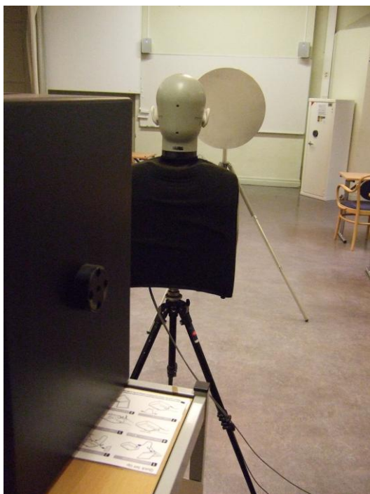
Fig. 1. Recording set up with the loudspeaker behind the artificial head and the reflecting object in front of the artificial head
