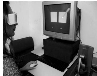
Figure 1. Experimental set-up. The computer screen with two targets, Phantom, 3D glasses and a mouse.
