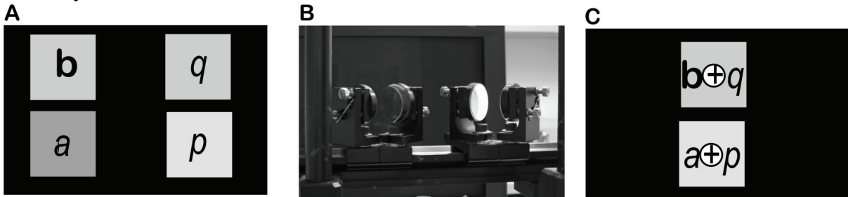
Fig. 1: Stimuli displayed on a monitor (A) viewed through a stereoscope (B), produce the subjective percept seen by the respondents (C). The a , b , p , and q values are luminance.
